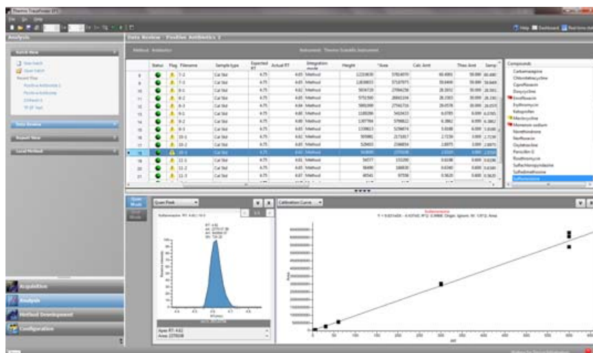
FIGURE 2. TraceFinder screen shot for the quantitation of the antibiotic sulfamerazine at 3 pg/mL
